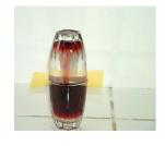
5.) We fill up a glass with water and another one with red wine. We cover the glass filled with water with a plastic plate and we turn it upside down. We can observe that the water does not run out because the pressure of the outside air presses the plate against the glass. Place the glass filled with water on the top of the glass filled with red wine and pull out the plate a bit. Wine and water switch places slowly because the density of wine is lower than the density of water.
